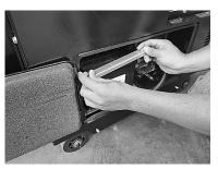
(2) Remove the battery terminal cover
