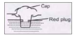
Overfill is dangerous. Do not fill the tank beyond the top of the red plug inside the fuel tank filter.
